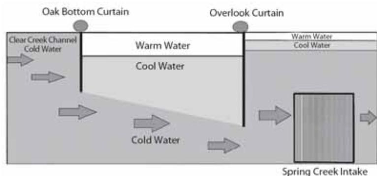
DIAGRAM 2 Thermally stratified water flow
