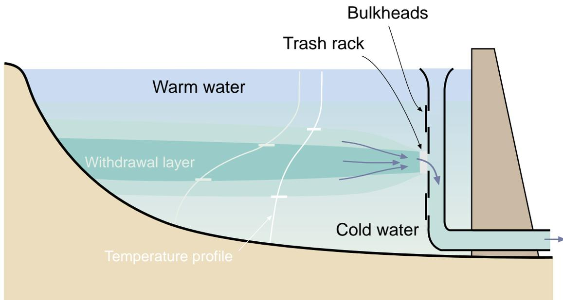
**Figure 1** Selective withdrawal removes water from strata within the water column. It is usually done by replacing one or more bulkheads in a multi-level outlet structure with trash racks to screen out large debris while allowing water to pass through the dam. The thickness of the withdrawal layer depends on the strength of the stratification and the discharge rate.
