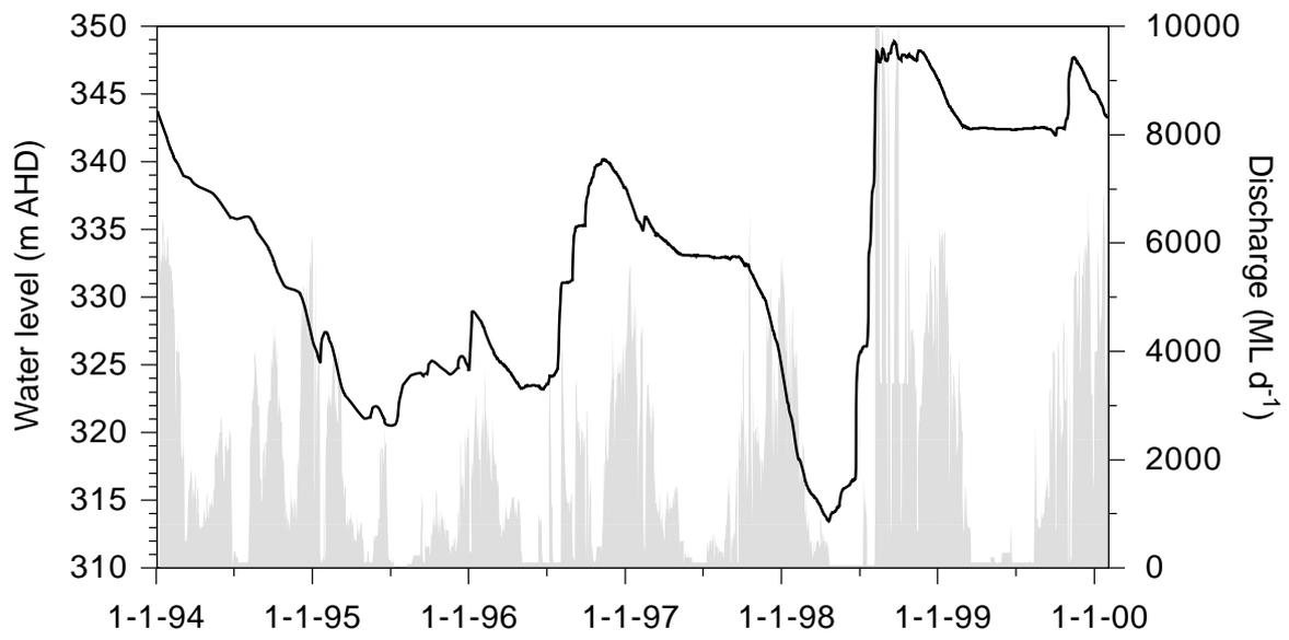
**Figure 8** Water surface elevation (line) and discharge (grey region) at Burrendong Dam.
