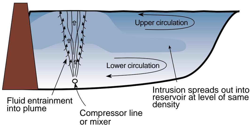
**Figure 2** Typical circulation pattern set up by artificial destratification.
