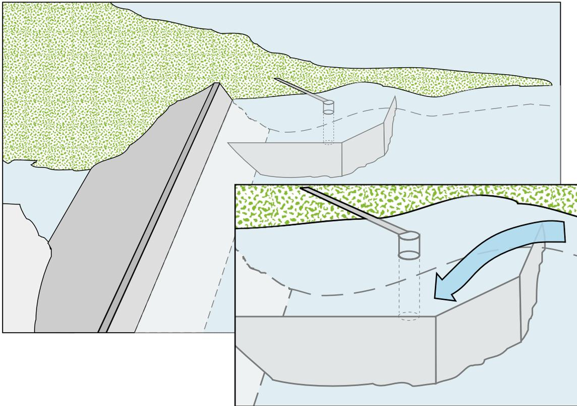
**Figure 7** Conceptual diagram of Burrendong dam, outlet tower and the proposed submerged curtain.
