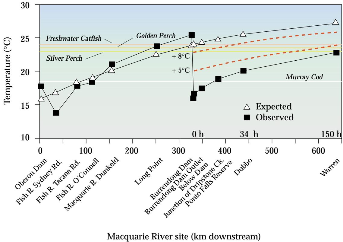
**Figure 6** Observed and expected river temperatures above and below Burrendong Dam. Also shown are the desirable spring-summer temperature requirements for successful spawning of several native Australian fish species (horizontal lines) and the projected river temperatures for increases in the discharge temperature of 5 and 8 °C (heavy dashed lines). Travel time under high flow conditions is 34 h from the dam to Dubbo and 150 h to Warren. Temperature data from Harris (1997).
