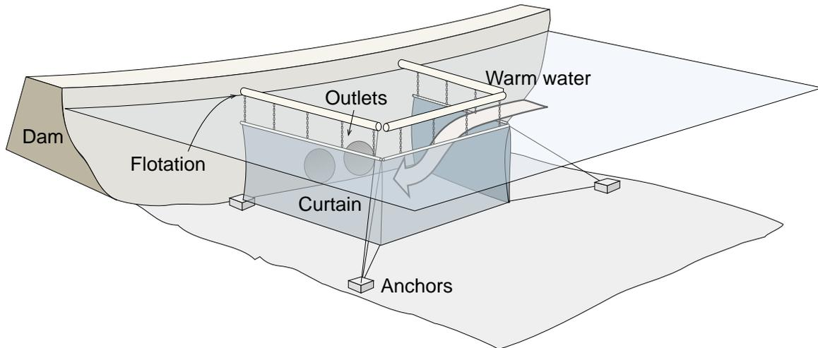
**Figure 5** A submerged curtain forces the release to originate from within the warmer surface layer of a reservoir.
