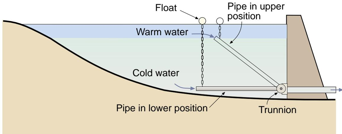
**Figure 4** A trunnion intake structure.
