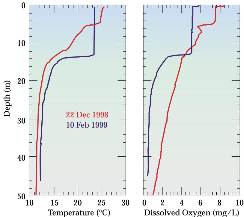
**Figure 9** Temperature and dissolved oxygen profiles during typical summer conditions at Burrendong Reservoir.
