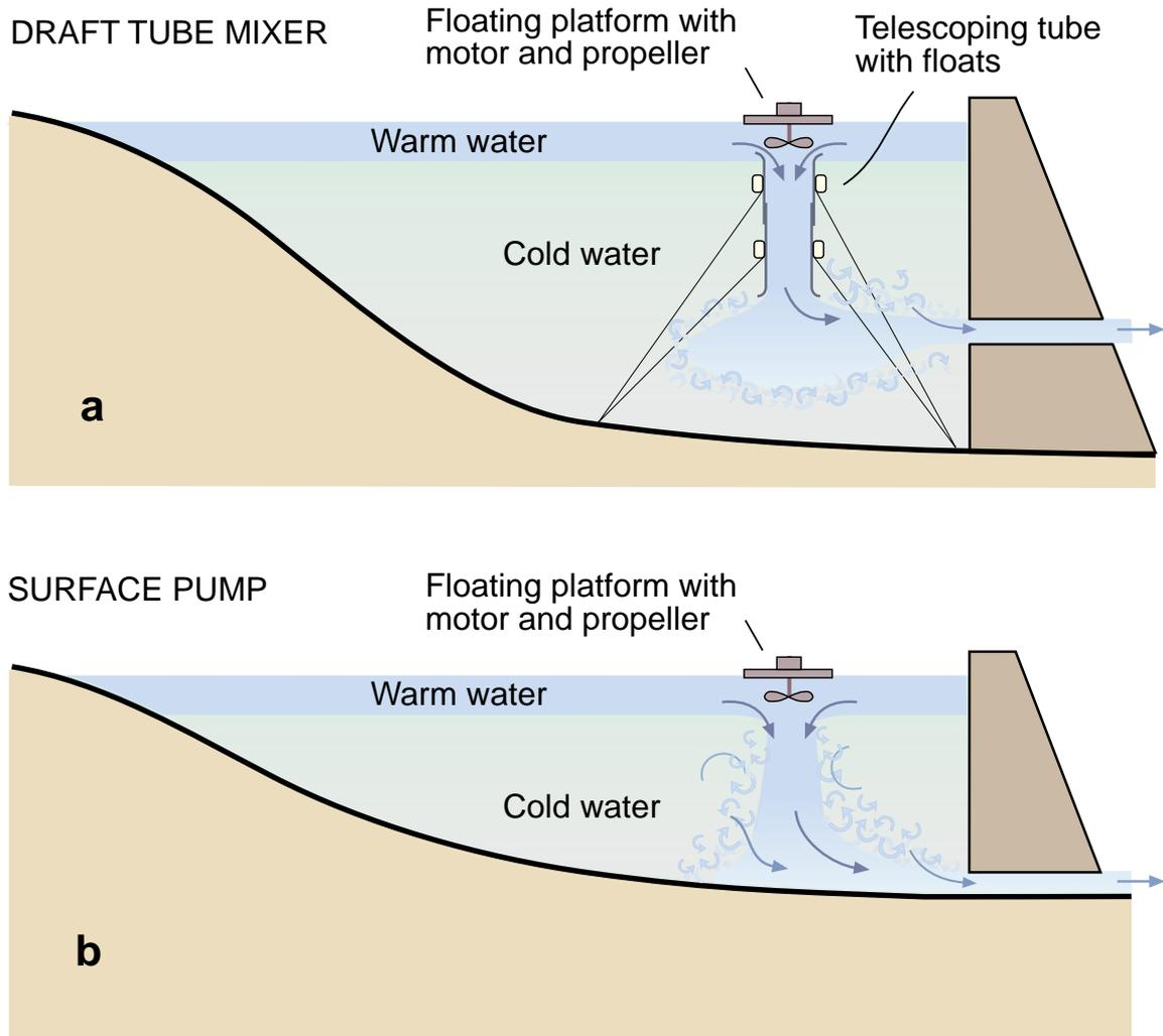
**Figure 3** Surface pumps send surface layer water downwards into the withdrawal layer adjacent to the outlet. a) The use of a draft tube decreases entrainment of reservoir water and can increase the energy efficiency of the system. b) An unconfined jet issuing from the surface pump is the simplest type of system to construct.
