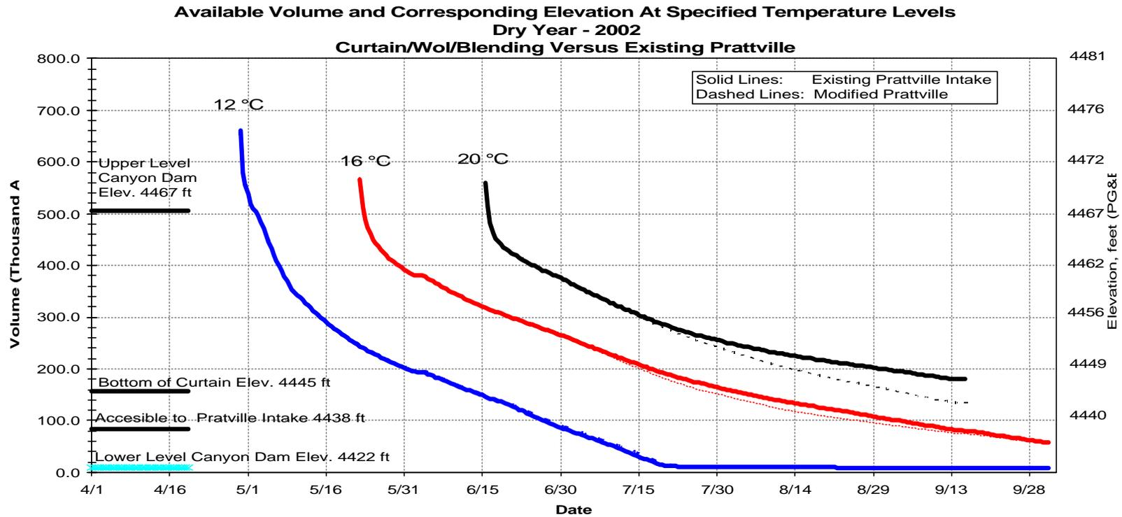
Figure 11A. Time Series of Volumetric and Corresponding Elevation Change for Three Specified Temperature Levels in Lake Almanor with and without Prattville Curtain for 2002, Operation in Dry Water Year Type
