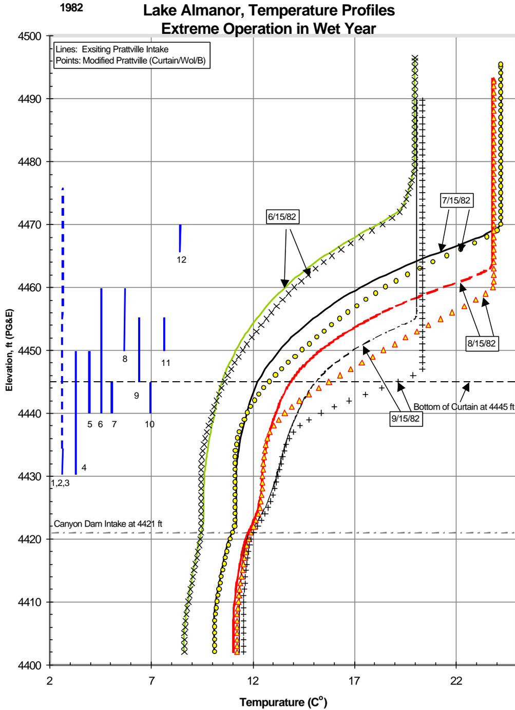
Note, blue numbered vertical lines (left side of figure) represent identified springs in Lake Almanor by elevation based on 1927 topographic map (PG&E datum). Location of vertical lines are not related to temperature axis.
