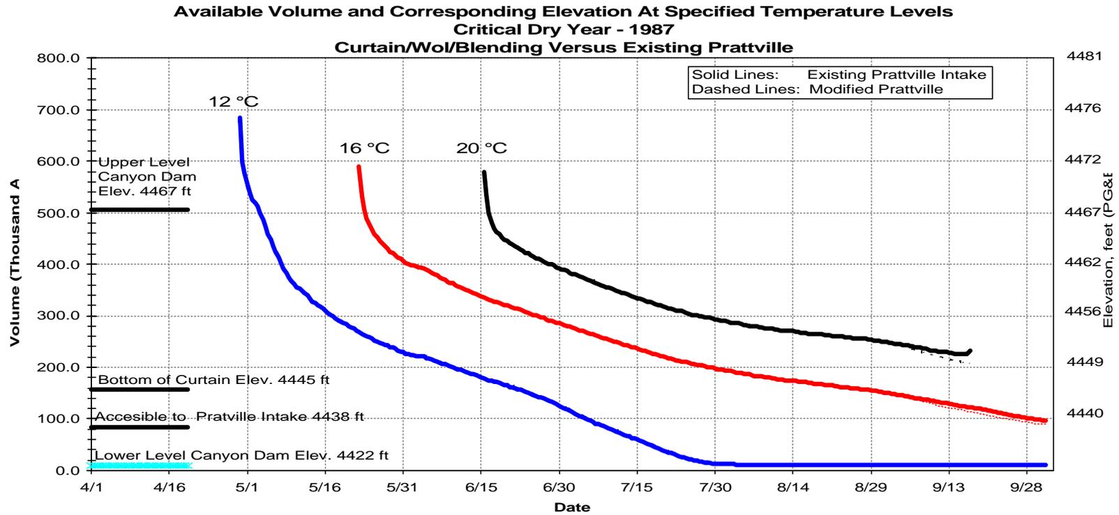
Figure 11B. Time Series of Volumetric and Corresponding Elevation Change for Three Specified Temperature Levels in Lake Almanor with and without Prattville Curtain for 1987, an Extreme Operation in Critical Dry Water Year Type.
